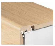
There is also an Incizo® solution for this. Simply turn around the aluminium sub-profile, so the short leg is resting on the stair tread. Cut off a part of the Incizo® profile with the Incizo® slitter. Stick the Incizo® profile onto its sub-profile. Ready!\*
