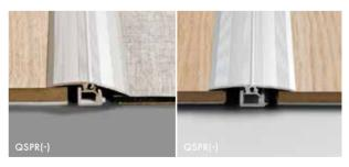
Profile in scratch-resistant aluminium to bridge height differences from 0 to 12.3 mm. To be used for instance between 2 Quick-Step laminate floors, or between a laminate floor and another lower or higher floor. Available in silver.
